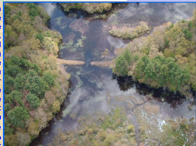
Arial photograph of the upper Regulating Reservoir that shows the aquatic plant growth in the northern part of the regulating reservoir. This can result from high phosphorous levels. Courtesy of Providence Water.
